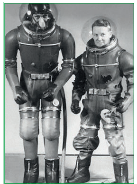
The "Tomato Worm," one of the few full-pressure suits developed during WWII for US Air Force pilots. – Credits: US Air Force
