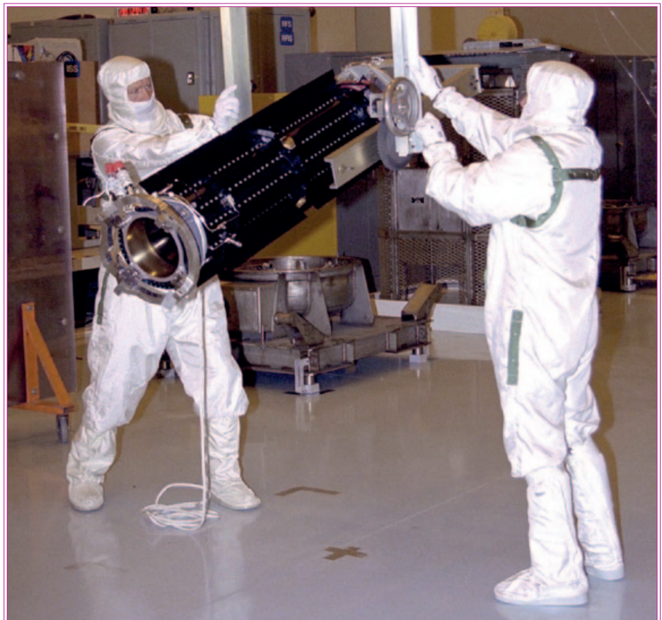
Jet Propulsion Laboratory workers handle a radioisotope thermoelectric generator (RTG) for the Cassini spacecraft mission to the Saturnian system. - Credits: NASA/JPL
