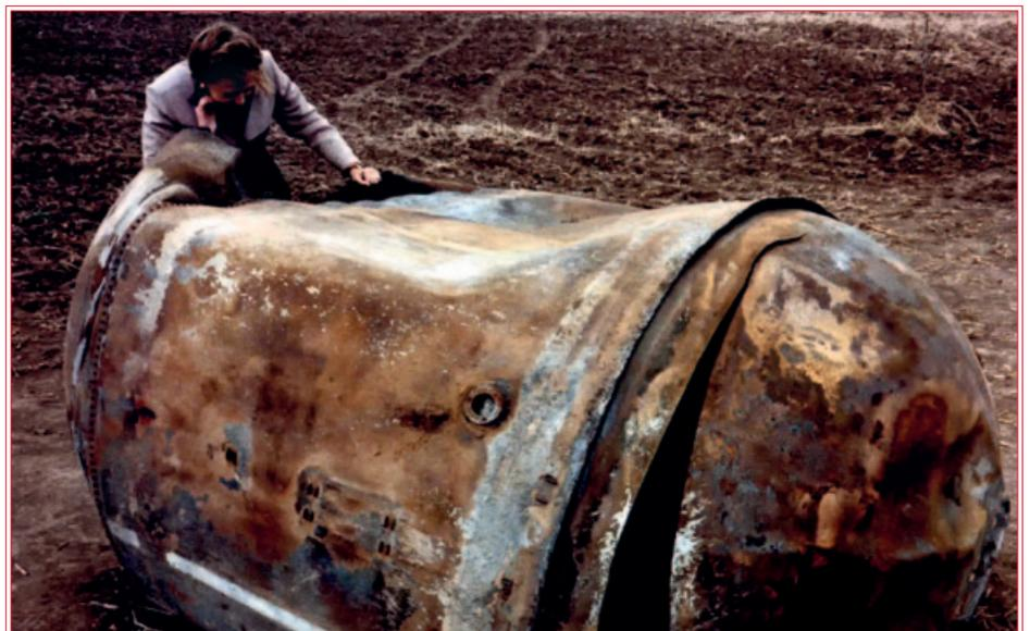
Recovered propellant tank from a spent Delta 2 second stage that survived atmospheric entry. – Credits: NASA
