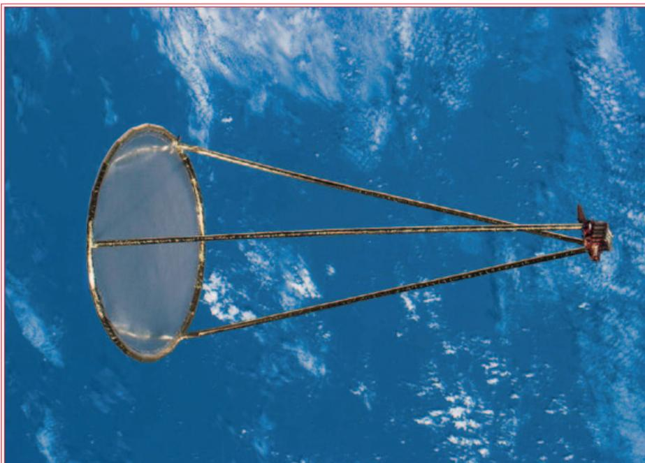
The Inflatable Antenna Experiment of May 1996 in deployed configuration.
