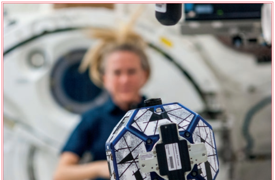
Synchronized Position Hold, Engage, Reorient, Experimental Satellites, or SPHERES, may not be humanoid but that doesn't mean they can't be helpful. These bowling ball sized robots are being used to perform environmental monitoring and maintenance aboard the International Space Station. – Credits: NASA
