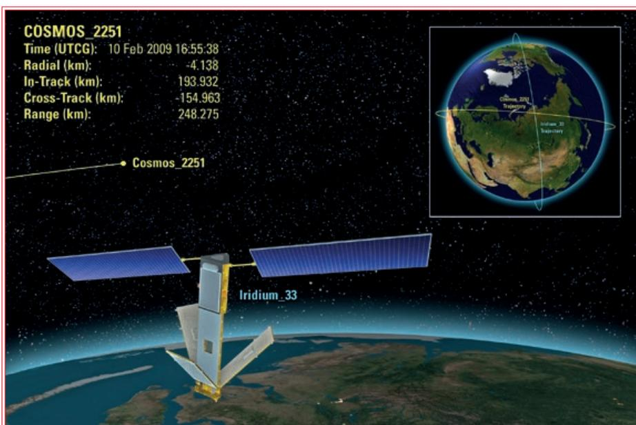
Illustration of the Cosmos-Iridium collision of 2009. The upper right plot shows trajectories of Iridium 33 (blue) and Cosmos 2251 (yellow) at time of collision. - Credits: Analytical Graphics, Inc. ([www.agi.com](http://www.agi.com))
