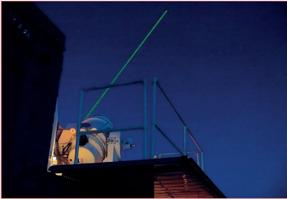
NASA's Satellite Laser Ranging Network uses lasers to measure distances from ground stations to satellite borne retro-reflectors to the millimeter level. – Credits: NASA
