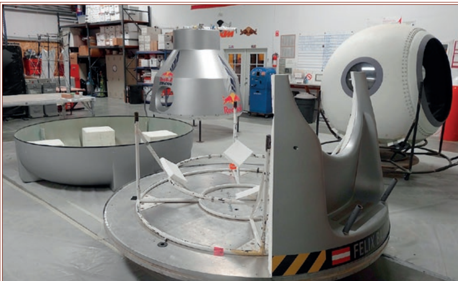
Red Bull Stratos capsule modular components: from left to right, the crush pad fairing, upper capsule and upper load frame, lower capsule section floor and load frame, and pressure sphere with bezel and hingeless door. – Credits: Sage Cheshire
