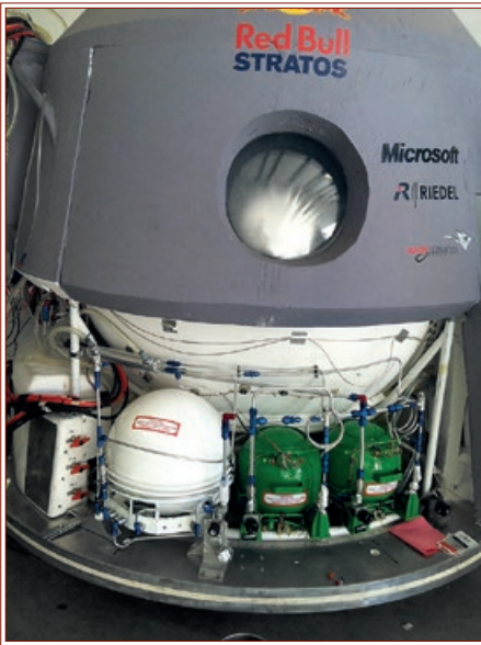
The Red Bull Stratos capsule with the temporary top cover before being loaded into the Brooks altitude chamber. Note the two 10 liter dewars of LOX and one 25 liter dewar of LN2 that are part of the capsule life support system. – Credits: Sage Cheshire
