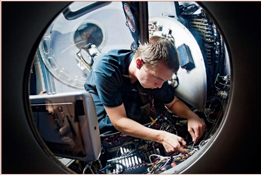
Jon Wells, Sage Cheshire Aerospace mechanical engineer and crew chief for the Stratos capsule, works to review the electrical system and instrument panel in the capsule before testing. – Credits: Sage Cheshire
