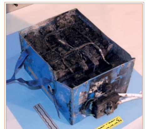
The JAL Boeing 787's APU battery involved in the Boston incident, on January 7, 2013.
