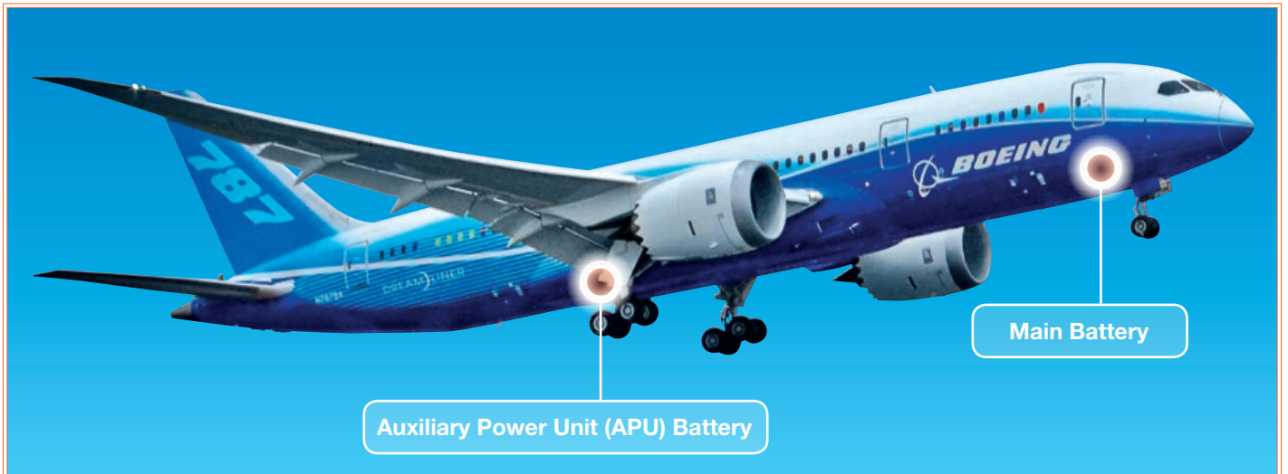
First flight of Boeing 787 Dreamliner on December 15, 2009. The Li-ion batteries are located on the 787 at fore and aft. – Credits: Dave Sizer
