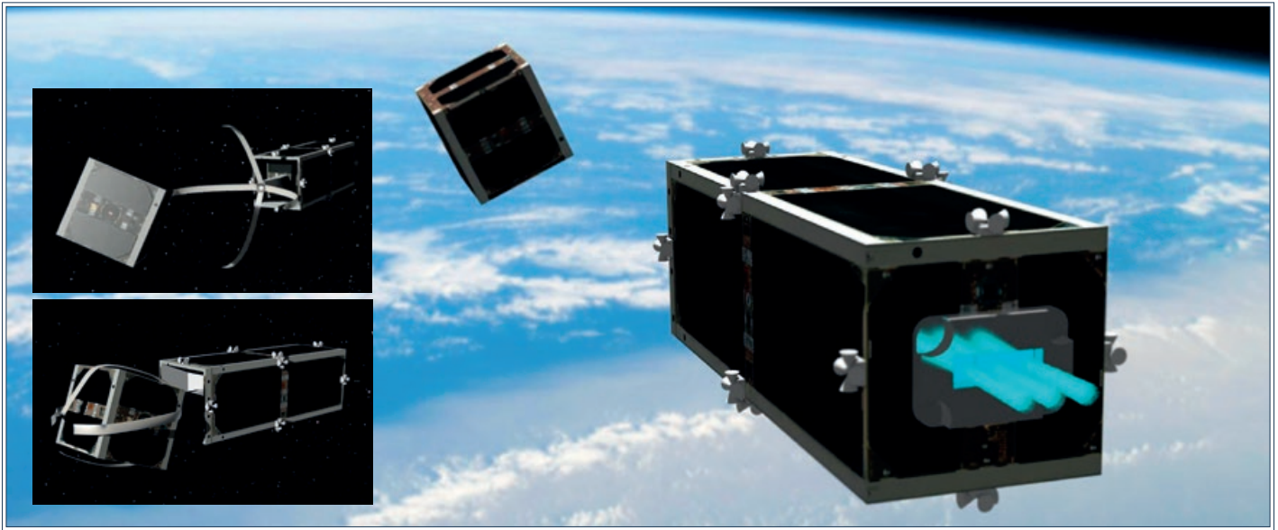
Artist's conception of CleanSpace One, a debris removal cubesat mission. – Credits: Swiss Federal Institute for Technology
