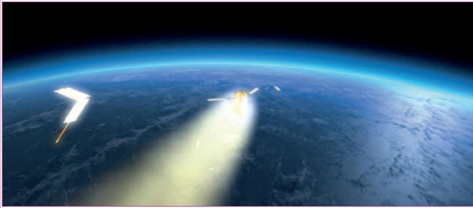
Artist's impression of an ATV spacecraft upon reentry. Controlled reentry over the open ocean greatly reduces the risk connected with falling debris. - Credits: ESA
