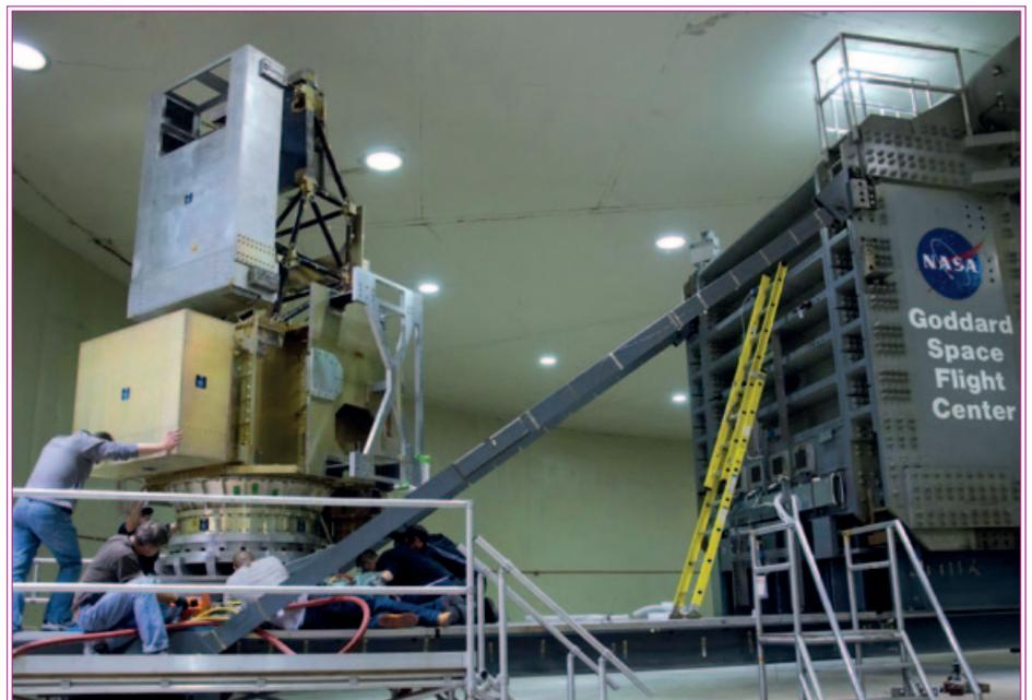
The Global Precipitation Measurement (GPM) satellite, under construction, is fitted to the bed of the High Capacity Centrifuge for spin testing. This spacecraft has undergone a "Design for Demise" overhaul. - Credits: NASA/GSFC
